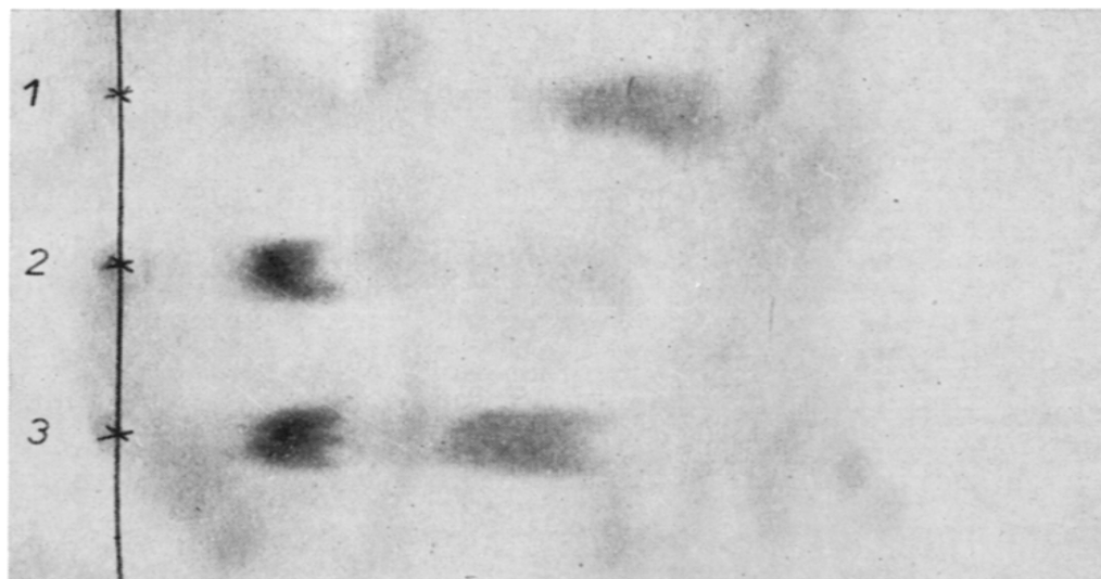
Fig. 3. Chromatogram of a separation of arsenite and arsenate ions. Solvent system: methanol-1 N \text{NH}_4\text{OH} (8:2, v/v), ascending. Length of run: 18 cm; 140 min at 20°. Detection: 2 N \text{AgNO}_3 in 10% ammonium hydroxide. As(III) gives a yellow spot, As(V) a brown spot; under U.V. light, blue absorbency. 1 = \text{Na}_3\text{AsO}_3 ; 2 = \text{Na}_3\text{AsO}_4 ; 3 = mixture of \text{Na}_3\text{AsO}_4 and \text{Na}_3\text{AsO}_3 .
